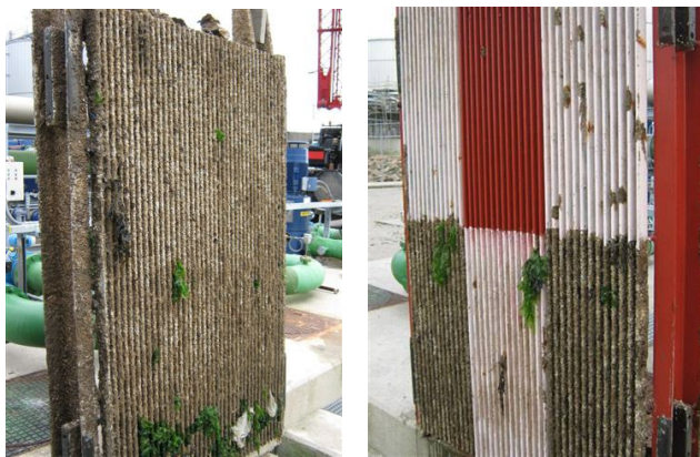
Figure 6 Test with different coatings, left non coated and right coated trash rack
