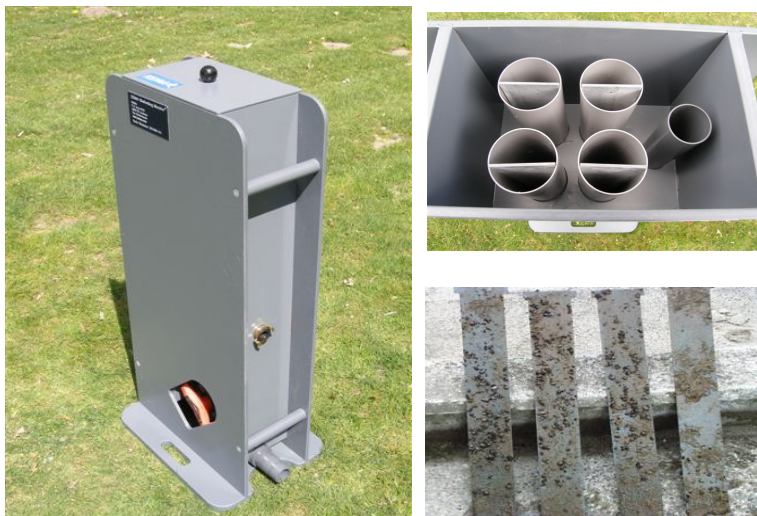
Figure 12 KBM, overview, top view and fouling plates which are placed in the monitor
